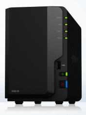
Synology DiskStation DS218 is a high-performance and versatile 2-bay NAS designed for small offices and home users to effectively manage, protect, and share data. Its 64-bit quad-core processor delivers high-speed data transmission and 10-bit 4K H.265 video transcoding to empower shared data storage and multimedia entertainment. Synology DS218 is backed by Synology's 2-year limited warranty.
